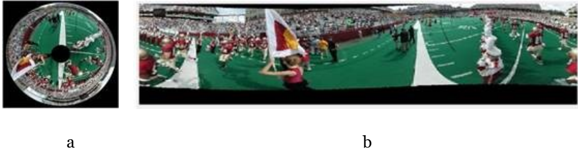
Figure 1 (a): Omnidirectional Image (b): Unwrapped equirectangular projection (ERP) Image
